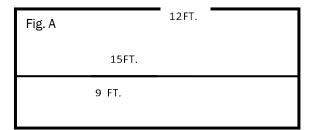
To verify that the working lines are square with each other measure 12' from the center point up the vertical length and make a mark. On the same horizontal quadrant line measure 9' across the width and make a mark, the diagonal measurement between the two marks should be exactly 15' if your lines are square. If your measurement is not 15' adjust your lines accordingly (see fig. A).
